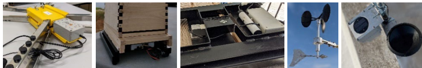
Fig. 9. IOHIVE end devices. a) BEEP base, b) SaveBees SMS scale, c) Kudzu scale based on Sprout, and d) MeteoHelix IoT Pro weather station MeteoWind IoT Pro wind sensor.
